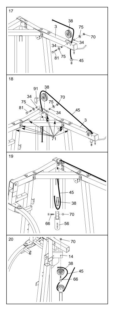
21. Wrap the High Cable (45) around a 90mm Pulley (38). Attach the Pulley at the forward hole, inside of the bracket on the Center Top Frame (14) with an M10 x 45mm Bolt (66) and an M10 Nylon Locknut (70).
